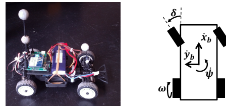
Fig. 9: RC car used for experimental results (left) with optical encoder, battery, radio modem, and reflective markers for motion capture. Diagram of car state (right) with body velocities \dot{x}_b and \dot{y}_b , heading rate \dot{\psi} , wheel speed \omega , and steering command \delta .
